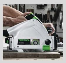
Integrated spring-loaded riving knife keeps the cut kerf open and the material away from the rear of the blade, reducing the chance of kickback and leaving the user in control.
