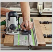
Designed for use with the FS Guide Rail system for guided cutting, MFS multi-routing templates, and a wide range of other accessory
