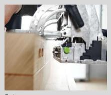
Quick and simple machining processes with the Domino Joiner provide the basis for rapid assembly of flat and corner joints utilizing Domino fasteners for knock-down design. Allowing for rapid building, moving, and reassembling of large pieces.
